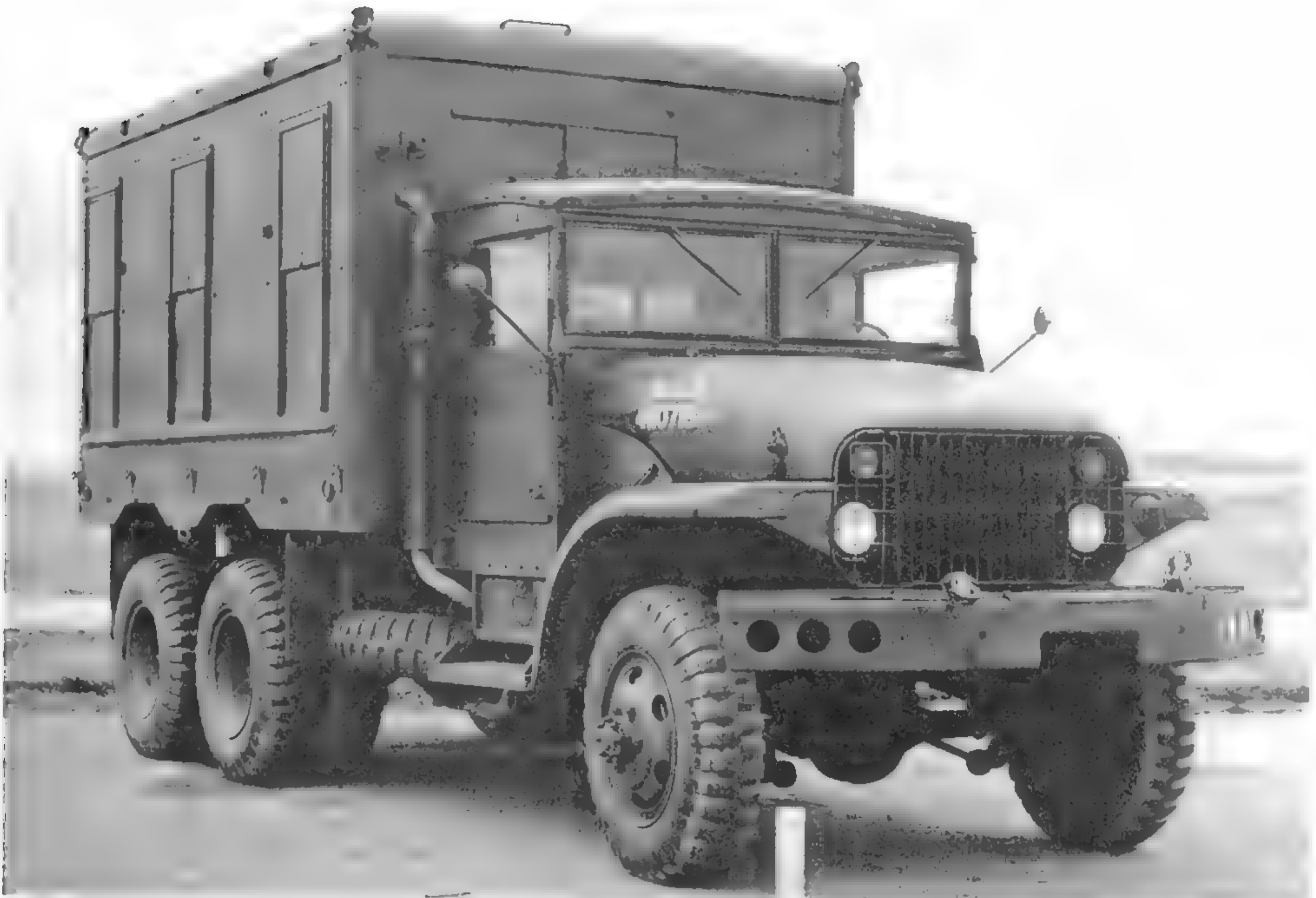
This M220 shop van was photographed at Aberdeen Proving Ground in January 1953. Supplied as an empty box, these could be fitted with a variety of repair-shop equipment loads, or with communications equipment. Access to the bed was through two unequal-sized doors on the rear of the body. (National Archives and Records Administration photo)
